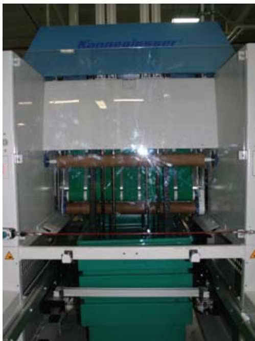
Another view of the sheet picker that separates textile goods before employees feed them into the ironer.
