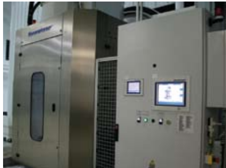
Above is a view of one of two tunnel presses in the plant. At right, an employee prepares clean textile goods in the plant's OR packroom for use in hospital operating rooms.
